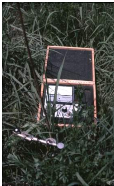
The quantum sensor measures PAR (photosynthetically active radiation) or visible light. The sensor is clamped to a pole at mid-canopy height in a prairie.
